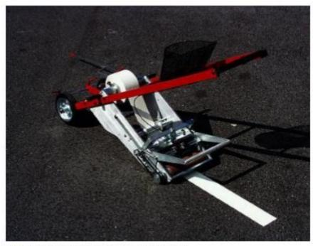
Figure 1: MTA-2 Tape applicator
